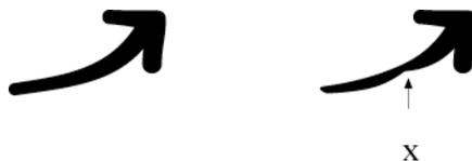
A narrowing of the clasp arm creates a point of flexure which weakens, and affects the flexibility of the clasp, since flexure begins at this point
