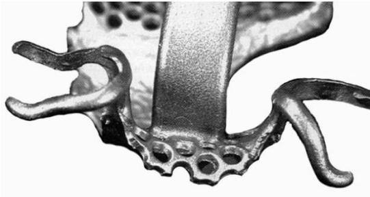
*Fig. 10. The metal framework of cast partial denture with sprues after shot blasting. (Markskors R. “Cast Partial Dentures”, 2000)*
