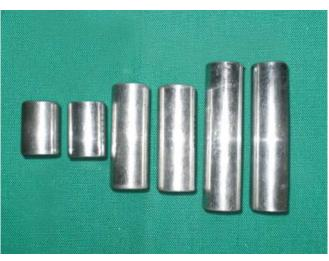
Fig. 1: Cartridges containing granules of flexible denture base material
