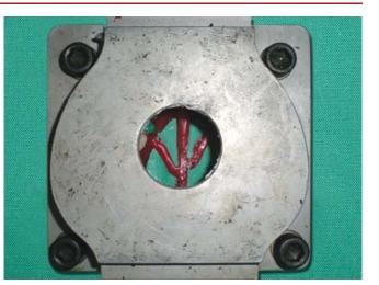
Fig. 3: Injection molding flask
