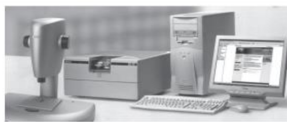
Fig. 13. Cerec inLab system – from left to right: inEos ekstraoral Cerec in Lab with inbuilt dot scanner, PC computer with 3D softver
